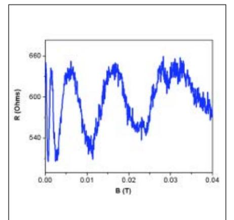
Figure 4. Resistance vs. applied magnetic field data of two MoGe wires in parallel showing oscillations. The period of oscillation is inversely proportional to the effective area enclosed by the two paths the electron can take, which decreases with increasing magnetic field. (Courtesy D.S. Hopkins)
