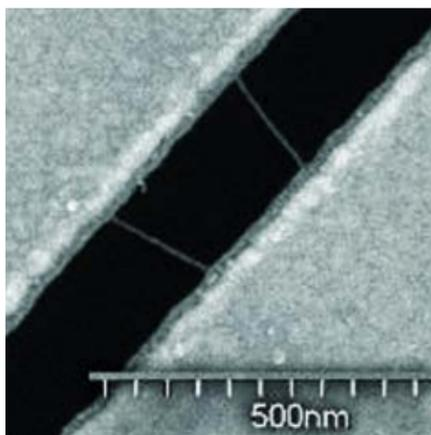
Figure 2. Scanning electron microscope (SEM) image of a pair of DNA wires. (Courtesy A. Bezryadin)
