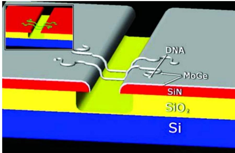
Figure 1. Diagram of a sample wafer with suspended DNA "bridges." The inset shows the strands of DNA suspended over an undercut trench in the substrate before sputtering. The sample is coated with MoGe, a superconducting metal, to make two nanowires.
