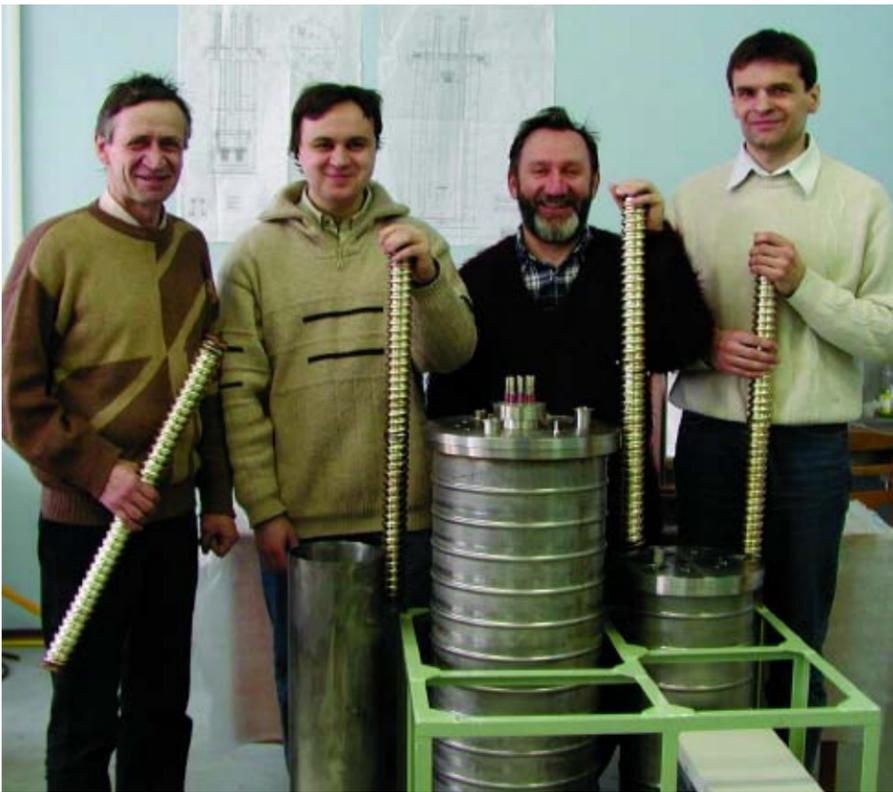
*Boris Bezymiannyh, Marat Vznuzdaev, Victor Trofimov, and Alexander Vassiliev from PNPI are shown holding the bodies of the adsorber-compressors of their novel hydrogen purification and handling system.*
