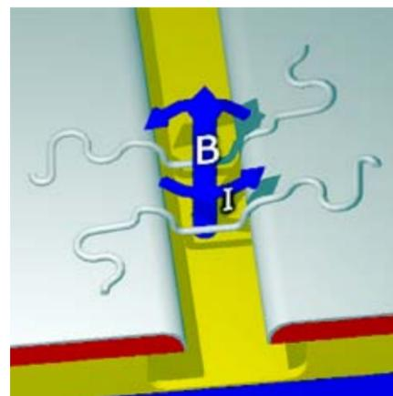
Figure 3. A strong magnetic field perpendicular to the wafer induces a current that flows in opposite directions across the pair of nanowires.
